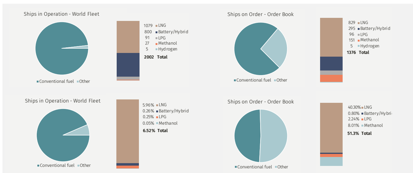
Figure 8. Alternate fuel uptake in the world fleet in number of ships (upper) and gross tonnage (lower), as of July 2023
